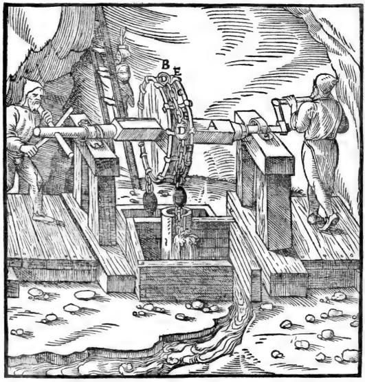
A-AXLE. B-DRUM. C-DRAWING-CHAIN. D-BALLS. E-CLAMPS.
